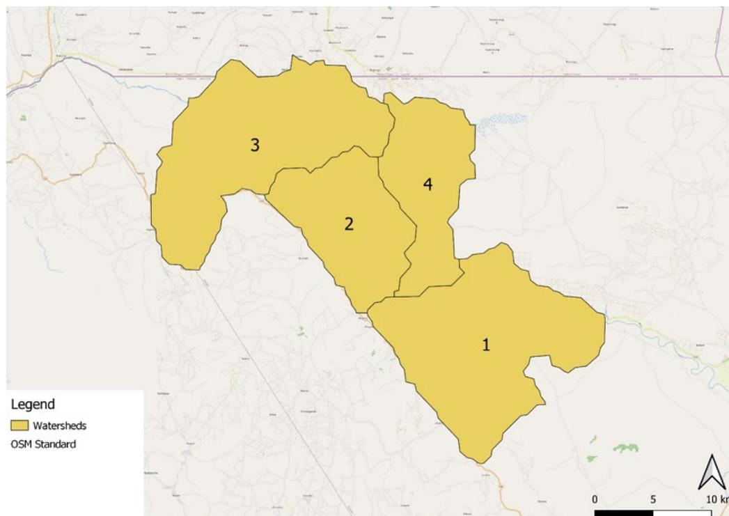
Table D7 shows that the reservoir created from the construction of the Kakono hydropower plant will increase water yield in almost all watersheds. In particular, the second one will experience a large increase in water availability (+14.51%), while in the third and fourth watersheds water volume will increase by 0.37/1.37%. The only exception is represented by the first watershed, where the volume of water yield will decrease by around 3%.
