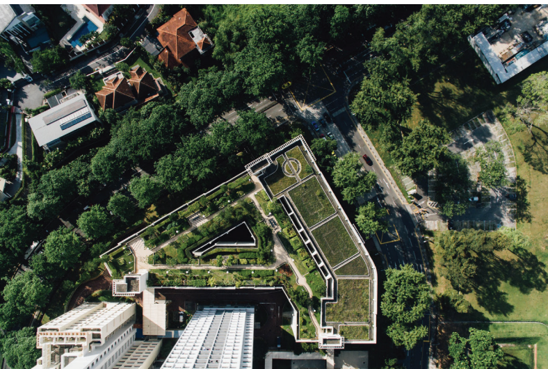
Green roofs, like this one in Singapore, reduce cities' heat island effect, decrease energy costs, improve air and water quality, sequester carbon, and provide habitat for urban wildlife. (Photo: CHUTTERS/NAP/Unsplash)
