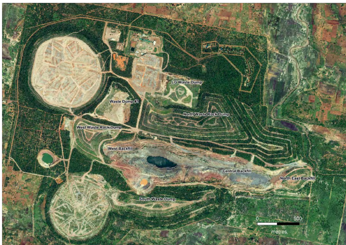
FIGURE 2. Surface layout of GPM in 2014, approximately 2 years after mining ended, showing the pit, waste rock dumps, and ring-dike tailings storage facilities
