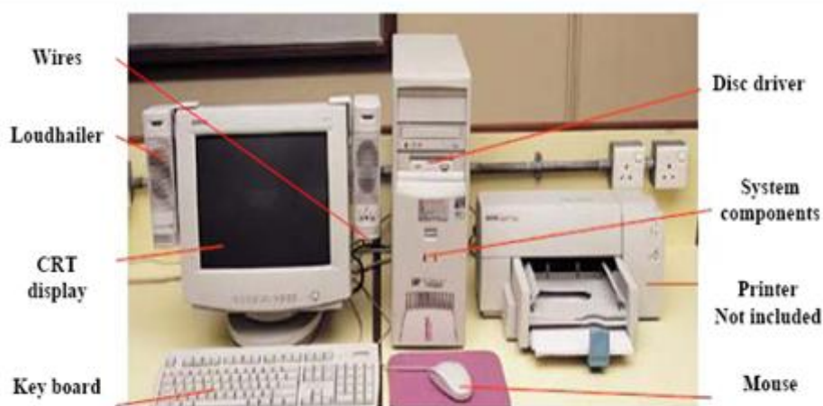
Figure 7: Functional unit of life cycle analysis—Desktop PC with CRT monitor, printer not included
