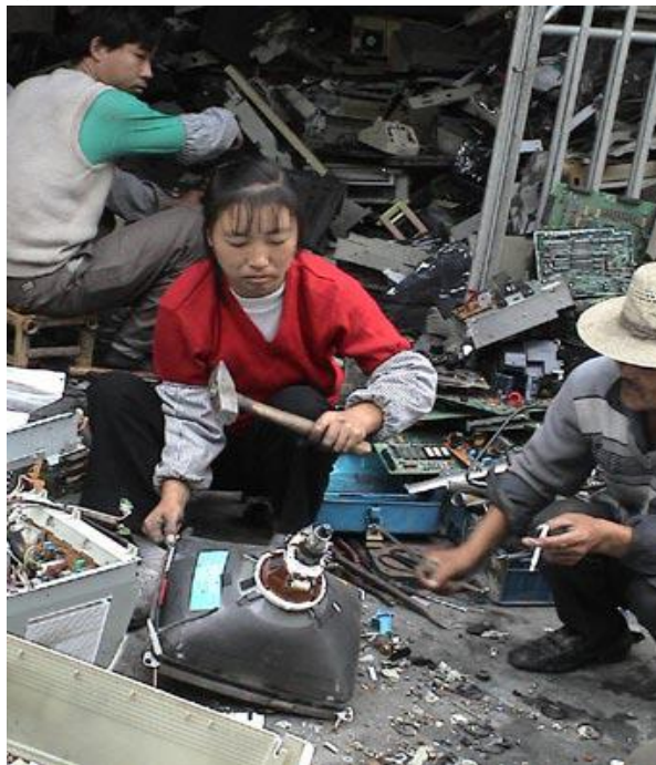
Figure 16: Unprotected dismantler cracking the yoke of a CRT screen. 14
