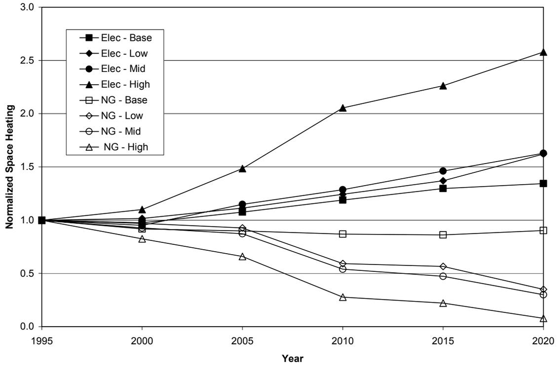
Figure 5: Normalized Space Heating Consumption: Electricity and Natural Gas
