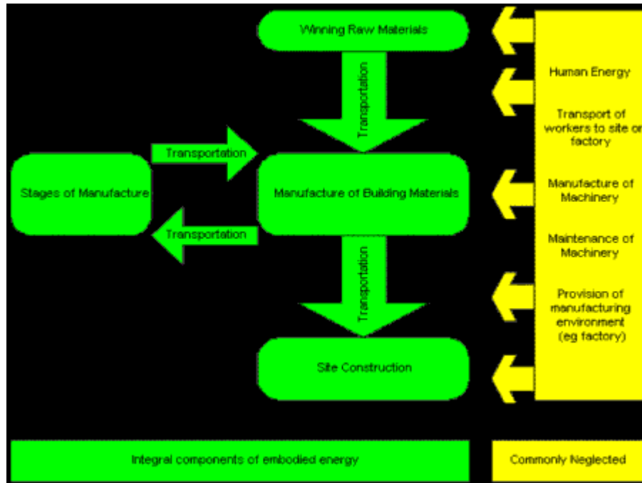
Figure 7-4. Components of embodied energy 15
