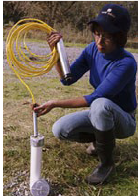
Figure 9. DWLR being deployed. Photo courtesy of Global Water.
