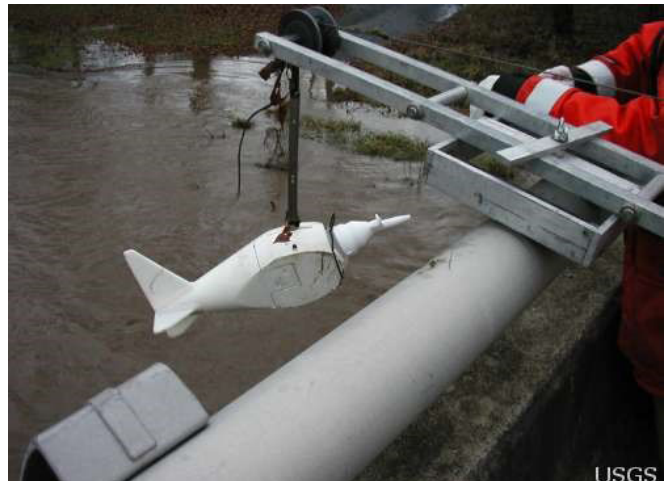
Figure 12. Deployment of the US DH-95 sampler. Photo courtesy of USGS
